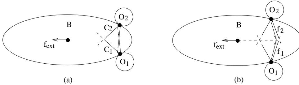
Figure 6.3: A frictional two-finger equilibrium which is (a) a non-resistant grasp, and (b) a wrench resistant grasp.
