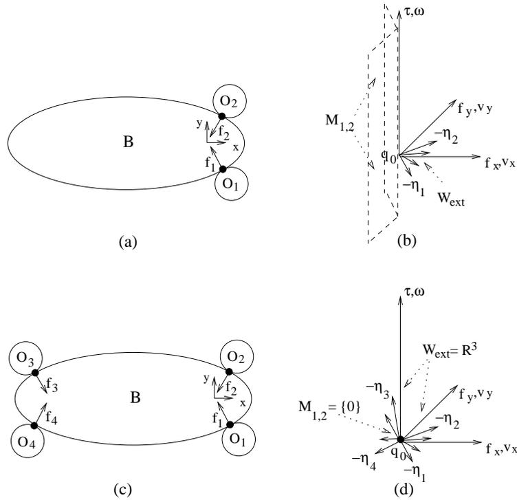
Figure 6.4: (a) A 2-finger grasp, and (b) the relation  $M_{1,2} = (\mathcal{W}_{ext})^*$  for this grasp. (c) A 4-finger frictionless equilibrium grasp which is (d) resistant and first-order immobilizing.
