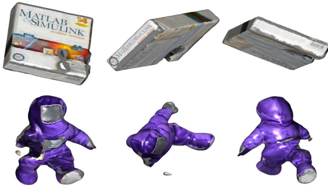
Fig. 9. Triangulated surface models constructed from surfel clouds. On the top is a Matlab box and on the bottom a stuffed doll. Any large holes are due to occlusion by the hand.
