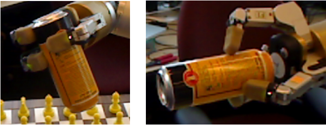
Fig. 3. Two grasps of the same object. With just a single grasp, the resulting object model will have holes. Between the two grasps, the entirety of the object is visible.
