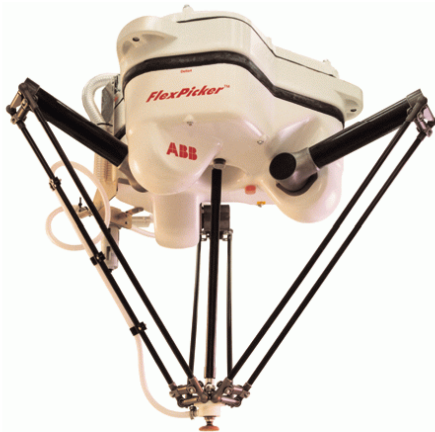
ABB Flexible Automation's IRB 340 FlexPicker (courtesy of ABB Flexible Automation)
