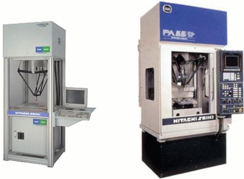
Hitachi Seiki's Delta robots for pick-and-place and drilling (courtesy of Hitachi Seiki)
