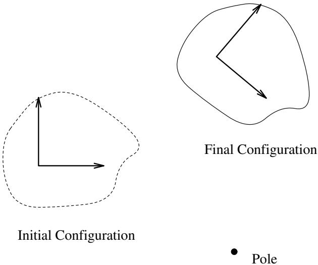
Let  $A$  be a fixed reference frame. A rigid body,  $L$ , which has local frame  $B$  attached to it, is located relative to reference frame  $A$  by  $D_1 = (R_{01}, d_{01})$ . Body  $L$  moves to position  $C$ , where the displacement to location  $C$ , as measured by an observer in frame  $B$ , is given by  $D_2 = (R_{12}, d_{12})$ .
