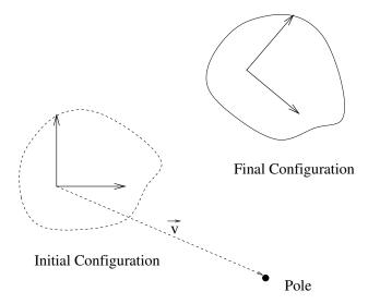
Let A be a fixed reference frame. A rigid body, L, which has local frame B attached to it, is located relative to reference frame A by  $D_1 = (\vec{d}_{01}, R_{01})$ . Body L moves to position C, where the displacement to location C, as measured by an observer in frame B, is given by  $D_2 = (\vec{d}_{12}, R_{12})$ . Where is the *pole* of the body displacement from position B to position C, as a function of  $R_{01}$ ,  $R_{12}$ ,  $\vec{d}_{01}$ , and  $\vec{d}_{12}$ ?
