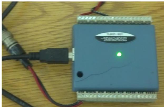
If an error message pops up, check that the DAQ has a solid green light. If the LED is blinking, disconnect the USB plug, and plug it in again.
